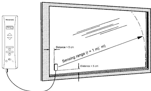
The additional function "broken glass indicator" requires an extra broken glass indicator for each **Vestamatic** Rollmat Plus G/S V3.1 roller shutter control (for larger or separated window panes). The installation of the sun sensor is described below.
